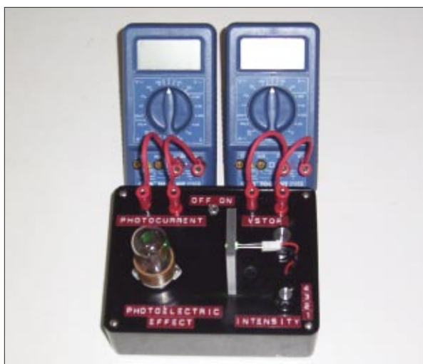
Fig. 1. The apparatus used for demonstration of the photoelectric effect. The light shield has been removed to show the phototube and LED. It is not required if the apparatus is used in a darkened room.
