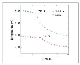
Fig. 2. Cooling curves for the iron and nickel spheres. The change in the slope occurs when the sphere jumps off the thermocouple and onto the magnet, indicating the corresponding Curie temperature (horizontal lines).
